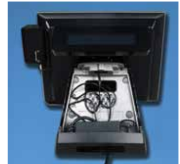
Cable Management Keeps Cords Hidden and Organized Neatly Tuck the Power Supply Inside the Cabinet
